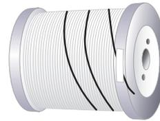
Attach wire to spool flange with tape.
